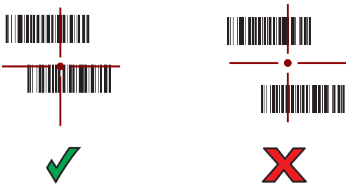
Figure 20 RS5100 Pick List Mode with Multiple Barcodes in Aiming Pattern
