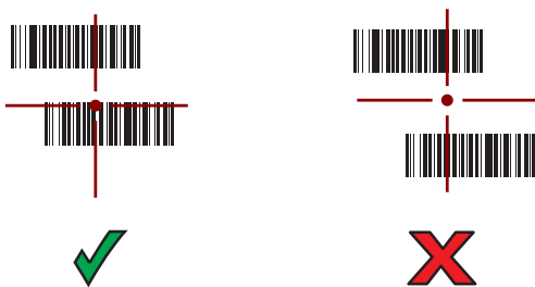
Figure 18 Pick List Mode with Multiple barcodes in Aiming Pattern
