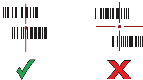
Figure 16 Pick List Mode with Multiple barcodes in Aiming Pattern
