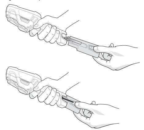
5. Press the battery into the handle until it snaps into place.
