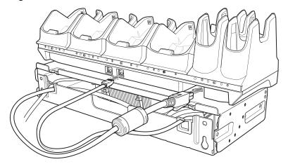
11. Secure top tray to bottom tray with 4 M5 screws (two on each side).
