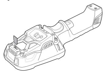
4. Align the bezel onto the device.
