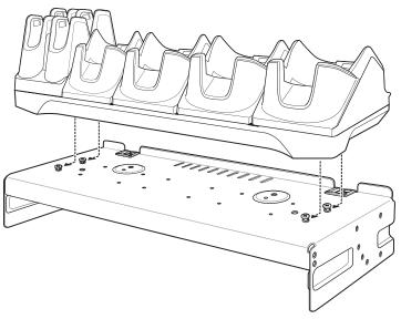
8. Secure cradle to top tray with two M2.5 safety screws.
