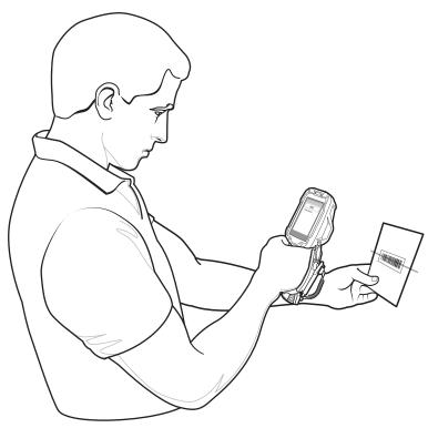
3. Press the trigger button. Ensure the red scan beam covers the entire barcode. The Charging/Scan LED Indicators illuminate green and a beep sounds to indicate a successful decode.
