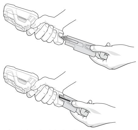
3. Press the battery into the handle until it snaps into place.
