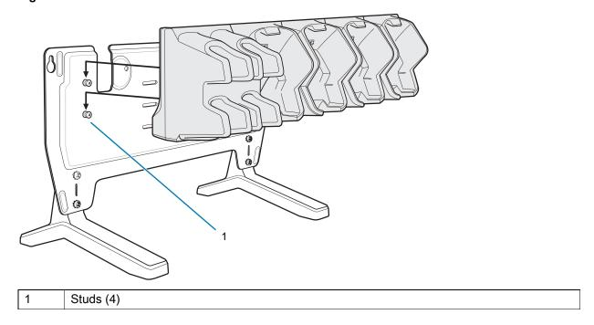
2. Secure cradle to plate using two safety screws.
