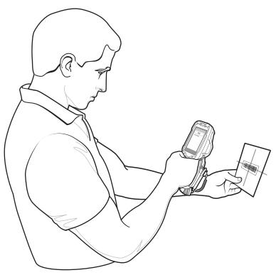
**4.** Ensure the red scan beam covers the entire barcode. The Charging/Scan LED Indicators illuminate green and a beep sounds to indicate a successful decode.
