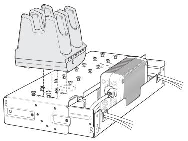
10. Connect DC Y cables to four 4-Slot Battery Chargers.
