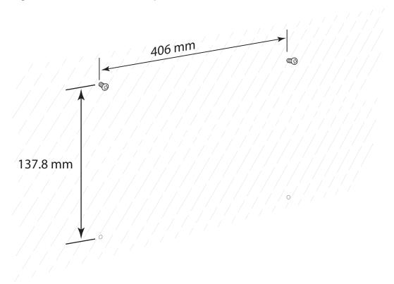
3. Align the mounting bracket's bottom mounting key holes with the screws.
