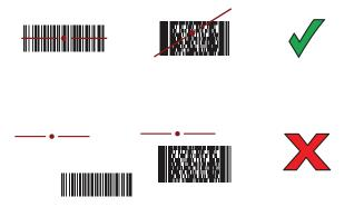
Figure 27 Imager Pick List Mode with Multiple Barcodes - Standard Range
