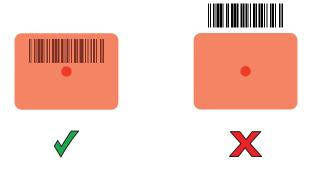
Figure 26 Imager Aiming Pattern - Extended Range
