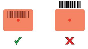
Figure 32 Pick List Mode with Multiple Barcodes in Aiming Pattern
