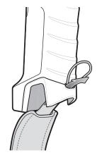
3. Insert the top end of the hand strap through the loop.
