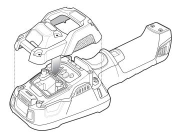
**6.** Secure Rear Bezel using six screws with a torque requirement of 4.5±0.2 kgf.cm.
