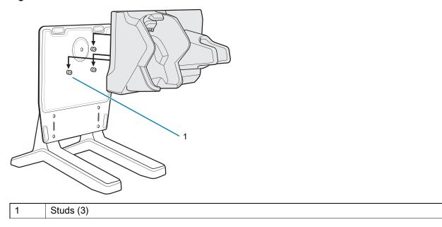
2. Secure cradle to plate using safety screw.
