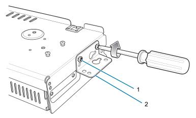
Figure 90 Flange 25° Position (4-Slot Battery Chargers)
