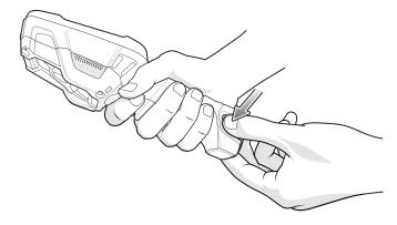
2. Pull the battery out of the device. The Charging/Scan LED lights red.
