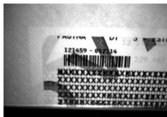
Figure 18 - Overprinted Barcode Readable by Matrix 120™ also Through the Envelope Window Film
